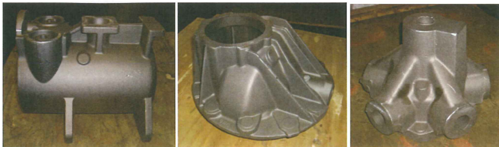
Fig. 9: Typical castings made in coal free greensand
