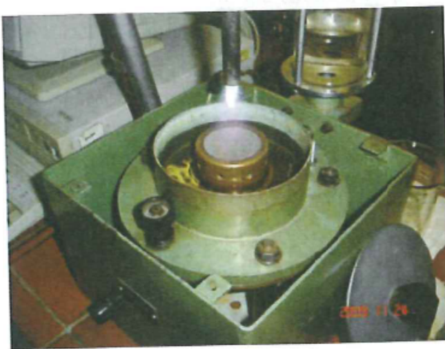
Fig. 6: The measurement of the stress from a heated greensand plate during flame heating. The total lack of coal increases slightly the stress, measured by the sensor under the plate
