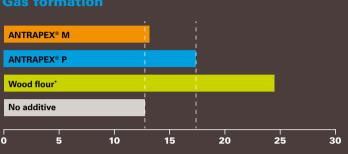
Gas formation, ml/g core sand (resin/hardener 0.8% each and 2% additive) \*Impregnated
