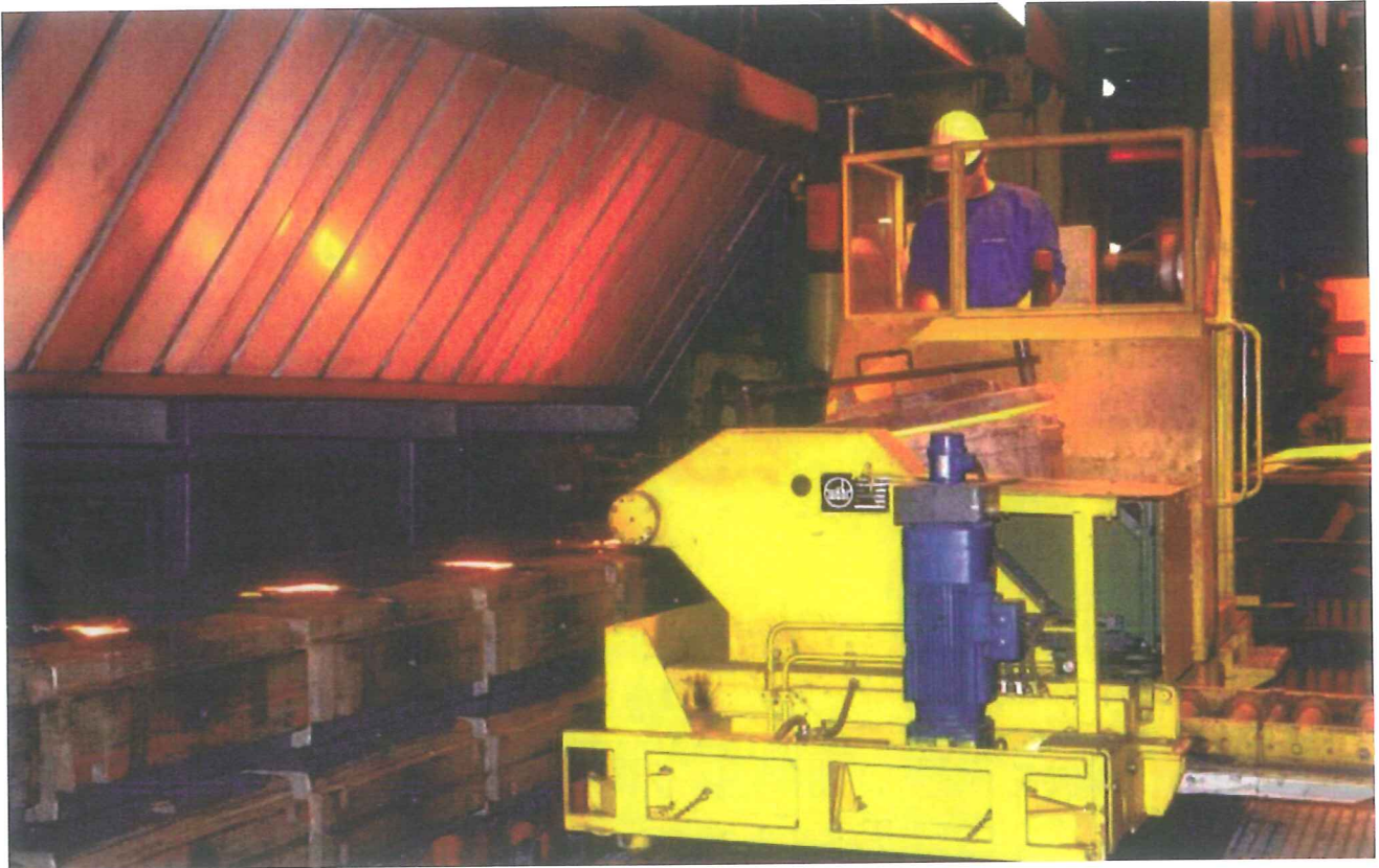
Pouring into molding sand without organic additives and without cores – no fumes are visible (Photos: S & B)
