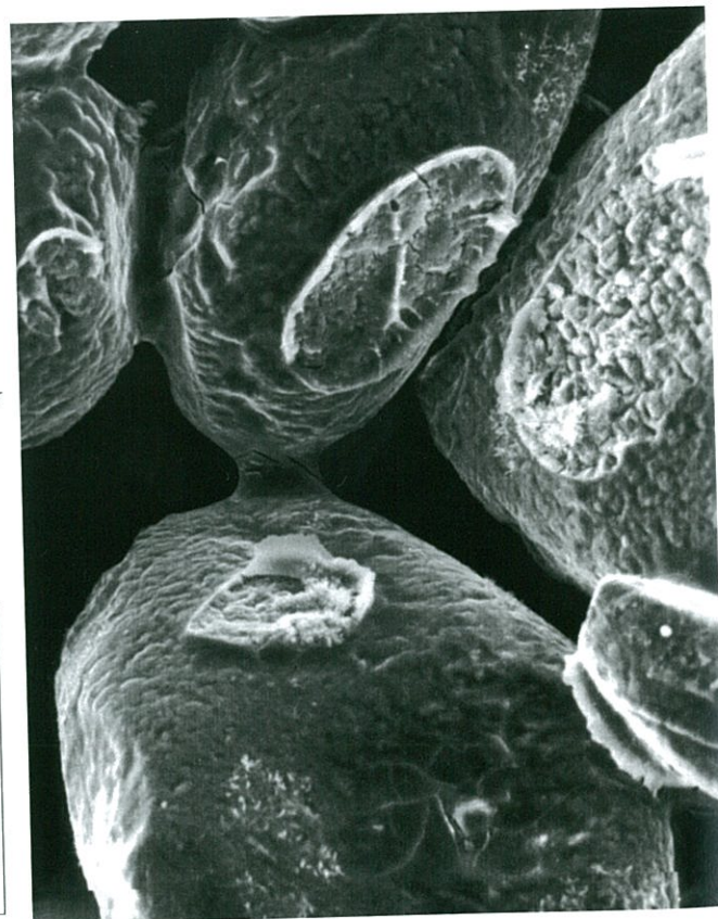
Figure 5. An example of a binder bridge with a lower tensile strength sodium silicate binder system on round grain silica.
